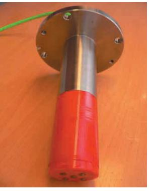
EML224SN-SA Sensor complete EML, 40m cable, for SIMRAD NL tank and gate valve.
